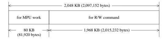
Figure 6.9 Data buffer configuration
